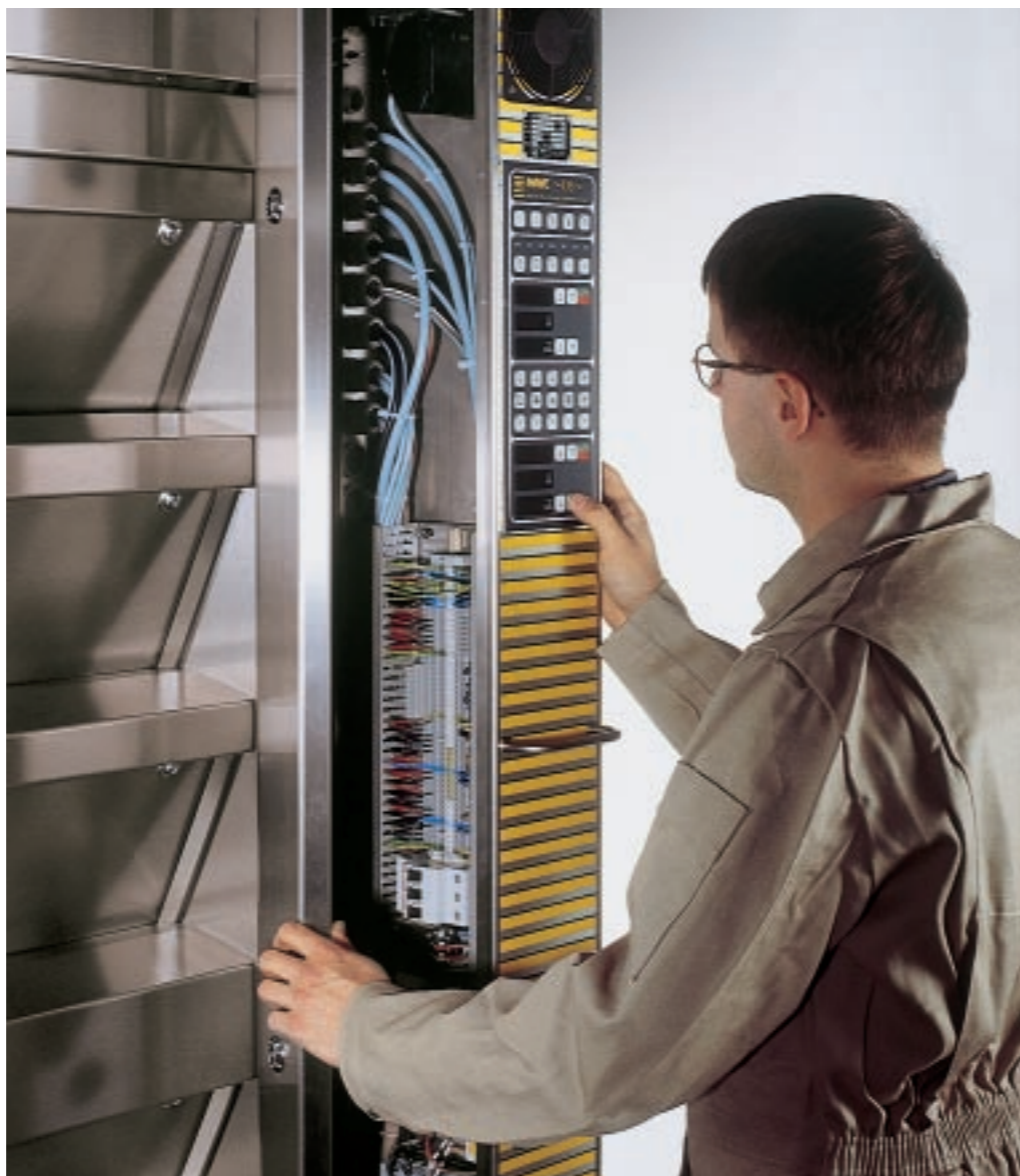
Removable oven control unit for easier maintenance
